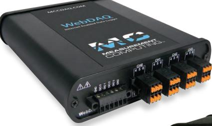
The **WebDAQ 904** Universal Input Logger features 4 universal inputs capable of measuring voltage (up to  $\pm 60$  V), current, thermocouples, RTD's, resistance, and strain gages.
